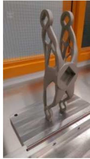
Figure 3: Physical printed part of optimized component
