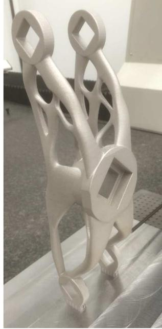
Figure 14: Real printed part using the Renishaw AM 500 metal printer
