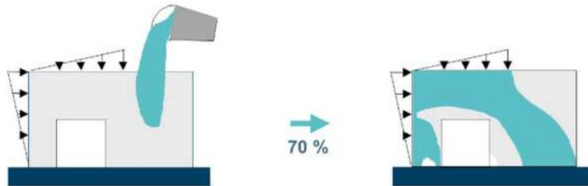
*Figure 4: The general goal of topology optimization is the distribution of material in a given design space. For the basic optimization task, the target mass is the constraint. For a given mass (target volume or target weight) the stiffness is maximized*
