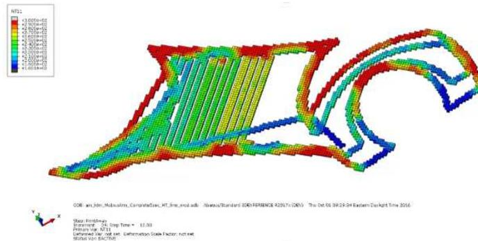
Figure 10: Detailed single layer finite element simulation results for a Mobius arm part with support and base
