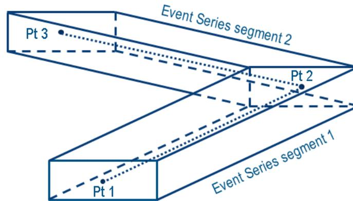
Figure 2: Event Series segments and moving boxes for element/material activation
