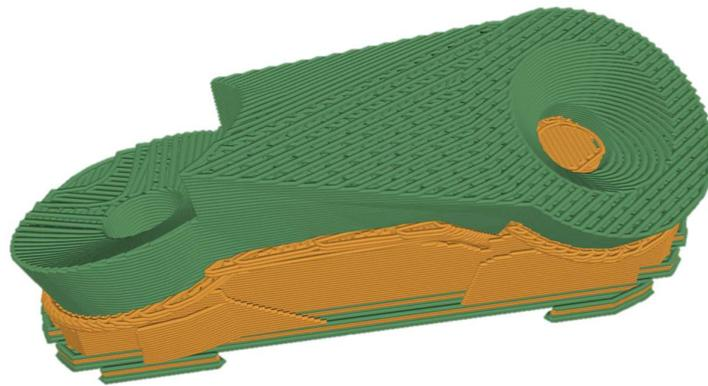
*Figure 7: Tool path generation for a Mobius arm part with support and base*
