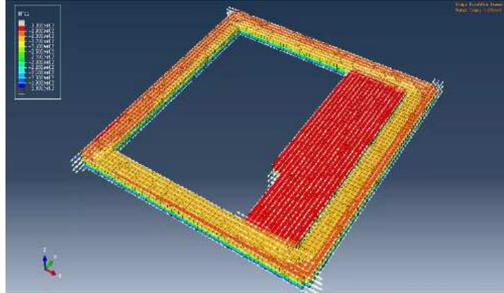
Figure 4: Material orientation assignment according to tool path data
