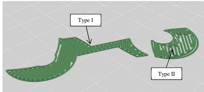
*a. Voids between contour and infill (type I); voids for partial infill (type II)*
