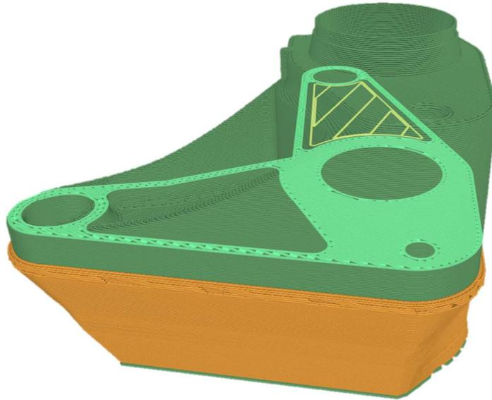
*Figure 1: Tool path generation for an aerospace rocker model with support and base*
