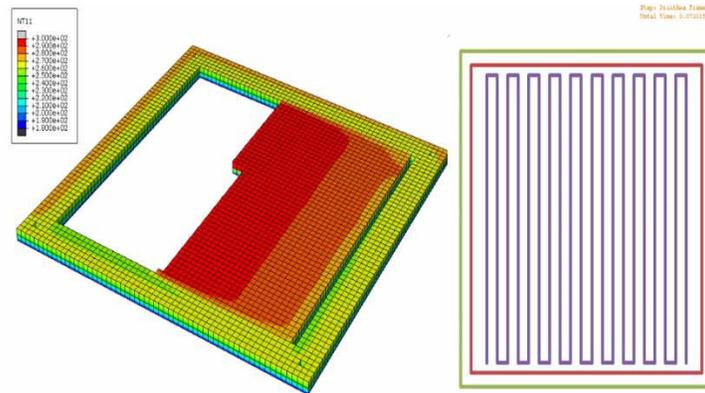
Figure 3: Element activation driven by tool path data
