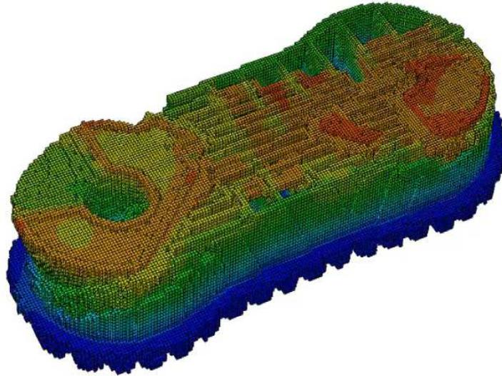
*Figure 8: Temperature result in the middle of the finite element simulation for a Mobius arm part with support and base*
