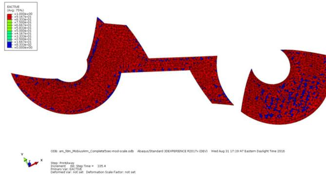
b. Type I and type II voids captured by the element activation algorithm
